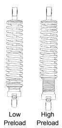
at least two turns of preload are holding the spring between the retainer on top of the shock and the threaded spring preload adjuster nut on the shock body.
